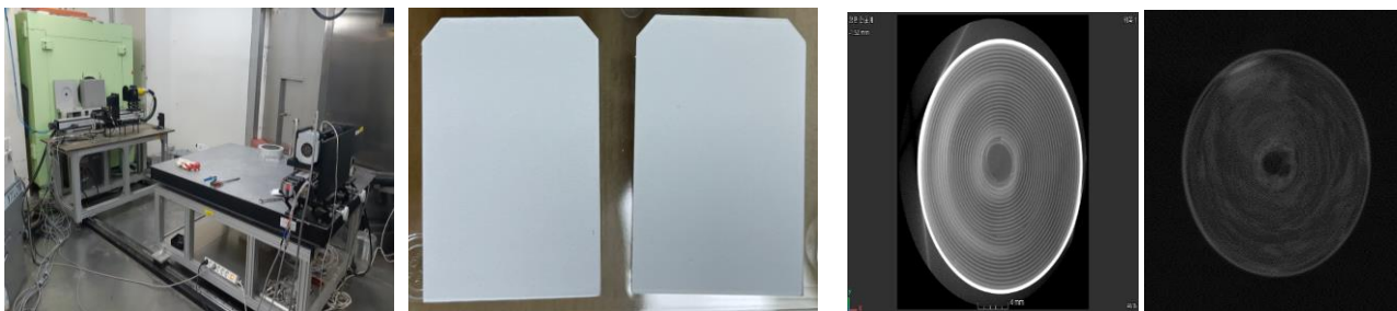
Figure 1. Picture of ENF experimental setup (left), Gd-based scintillating screens (center) and X-ray and neutron slice images with a cylindrical lithium-ion battery (right).
