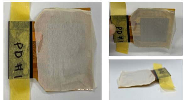
Fig.1. Images of CsPbBr 3 nanocrystal-PVDF nanocomposite scintillator film coupled F-PCB
