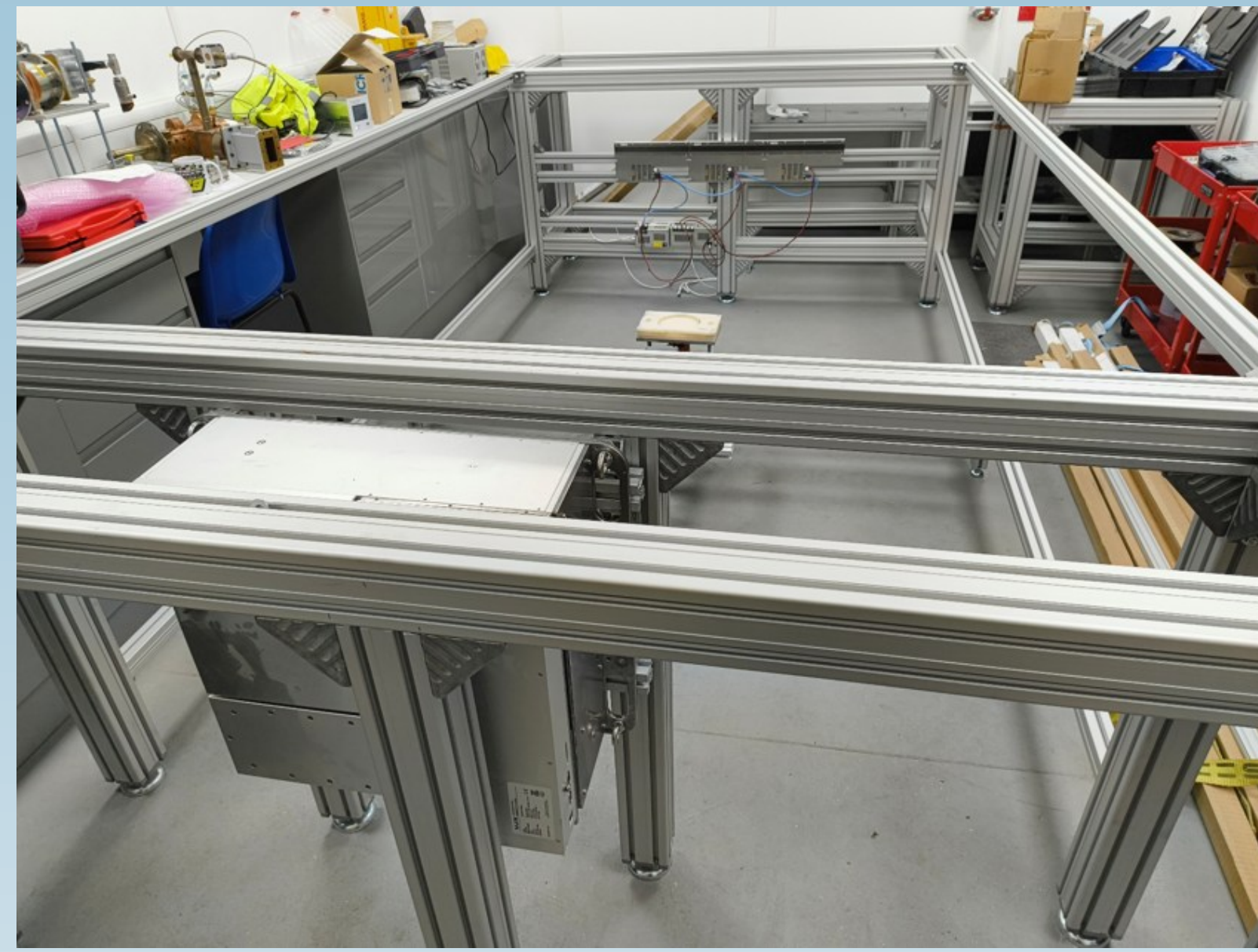
The combined system under construction at Rapiscan, combining a 320 keV X-ray tube (foreground) with LYSO scintillator array (background)
