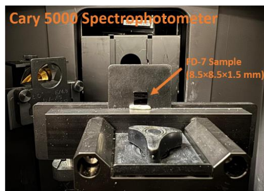
Figure 1 – Irradiated Flat FD-7 RPL sample under Cary 5000 spectrophotometer.
