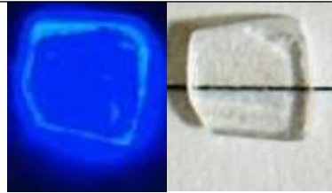
Photograph of Cs 3 Cu 2 I 5 SC under 254 nm UV lamp, and day light.
