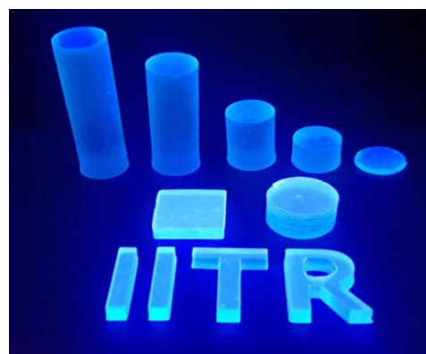
Fig.: 3D-printed scintillators under UV-illumination
