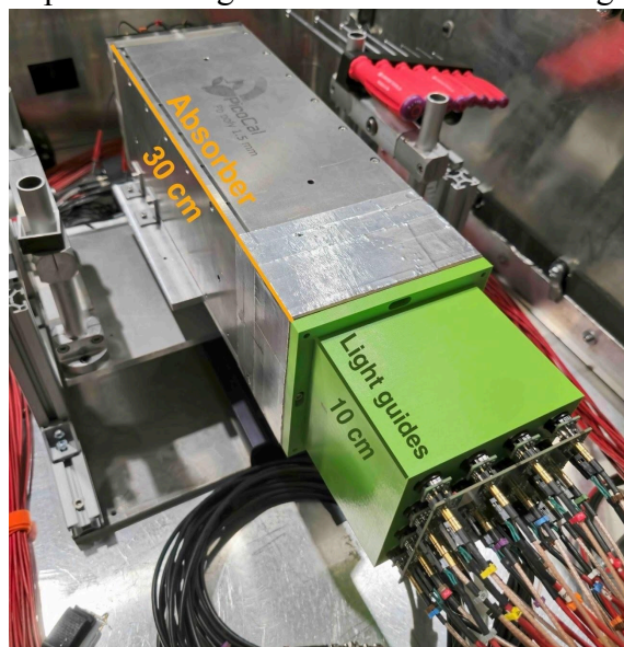
Picture of the SpaCal prototype with lead absorber, 3HF polystyrene fibres, and radiation-hard light guides.
