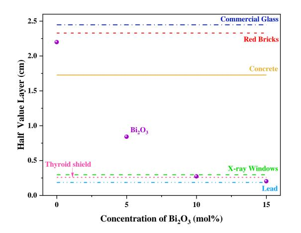
The glass samples Bi<sub>2</sub>O<sub>3</sub> 15 mol% compared with standard materials
