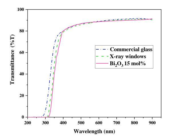
•The transmittance of glass samples Bi<sub>2</sub>O<sub>3</sub> 15 mol% compared with standard materials
