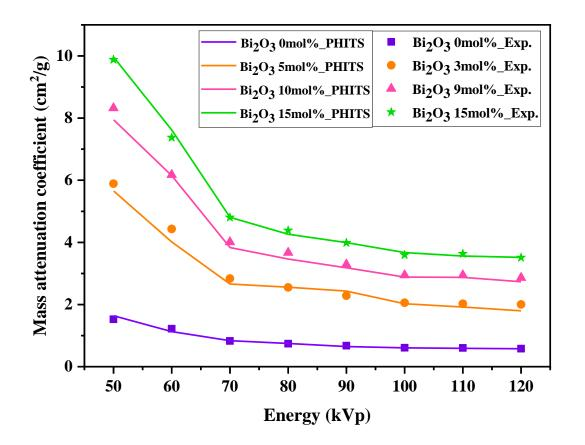
•When the concentration of Bi increases, the mass attenuation coefficient also increases.
