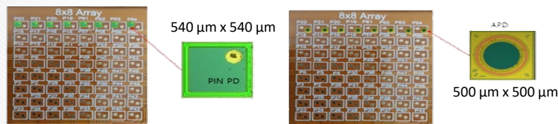
Images of F-PCB w. 64 ch. Si PIN and APD device installation
