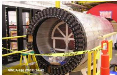
Start from mature layered Pb/ScFi technology with side-readout (same as the GlueX calorimeter) for state-of-the-art sampling calorimeter performance
