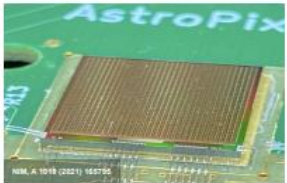
Insert layers of monolithic AstroPix sensors (inexpensive ultra-low-power silicon sensor developed for NASA) in the first half of the calorimeter to capture a 3-D image of the developing shower
