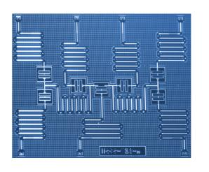
Superconducting circuit (초전도체 서킷)
