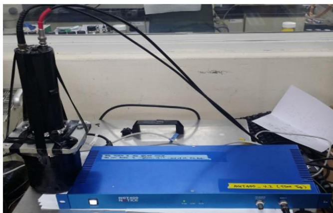
Figure 3.3: The photograph of LSC, PMT, and NGT400.
