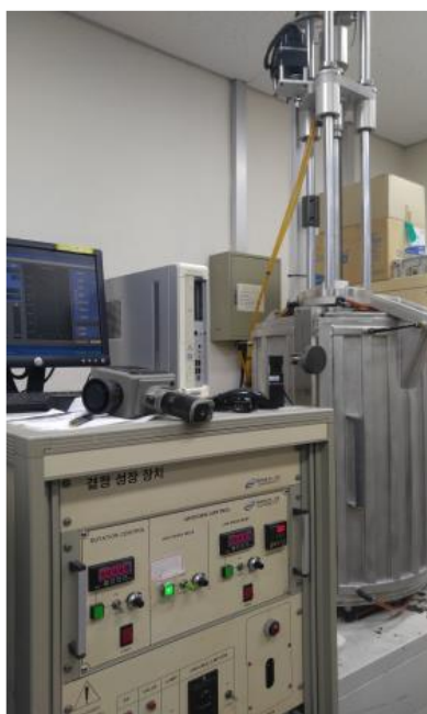
Figure 3.2.2. A photographic image of the Czochralski crystal growth apparatus.
