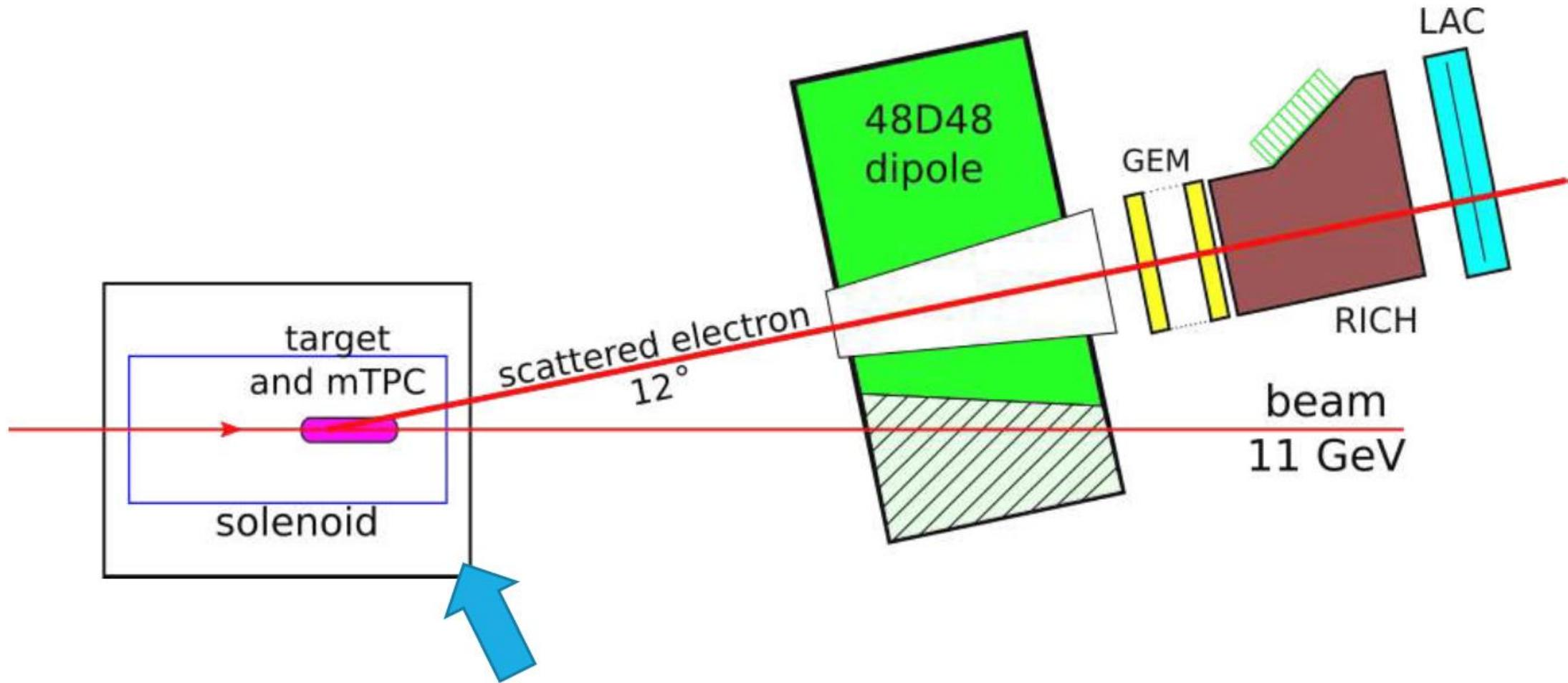
A new detector → mTPC: multi-Time Projection Chamber to measure low-momentum recoil protons
