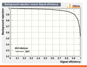
The ROC curve of a Boosted Decision Tree classifier indicating the high performance when identifying and removing charged particles contamination from neutron sample
