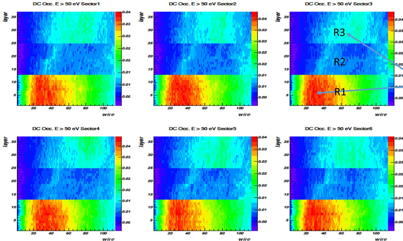
2 to 3 times higher occupancy in part of R1 than R3. Limits operating luminosity.
