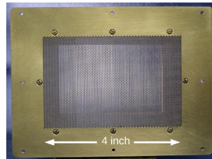
Figure 3: Active volume casing. Perforated area of  $L \times H = 4'' \times 2.626''$
