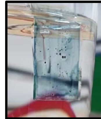
Demonstration of EC devices for smart window applications (NAPL)
