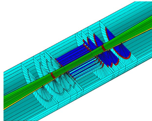
Figure 2: The vertex detector as simulated in ILCroot.
