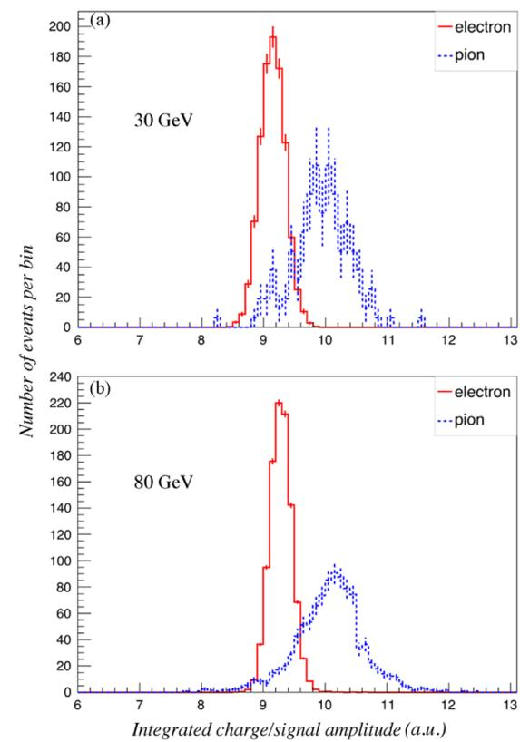
**Fig. 11.** Distribution of the ratio of the integrated charge and the amplitude of the signals produced by electrons and pions in one module of the RD52 fiber calorimeter. Data for 30 (a) and 80 GeV (b).
