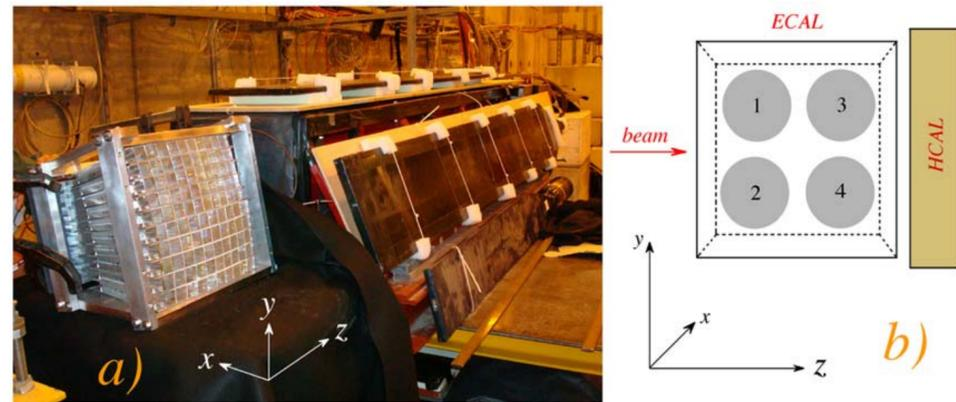
**Fig. 1.** The calorimeter during installation in the H4 test beam, which runs from the bottom left corner to the top right corner in this picture. The 100-crystal BGO matrix is located upstream of the fiber calorimeter, and is read out by four PMTs on the left (small end face) side. Some of the leakage counters are visible as well (a). The location and numbering of the PMTs reading out the BGO crystal matrix (b).
