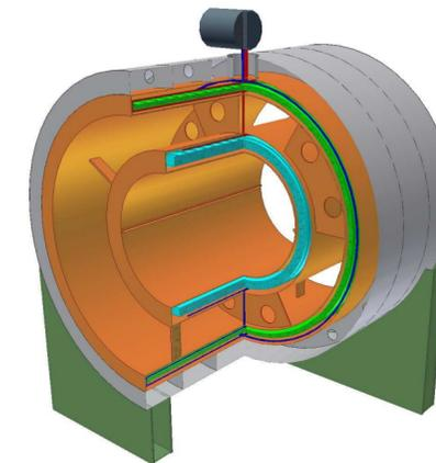
Figure 24: Cut view of the two solenoids and their supports.
