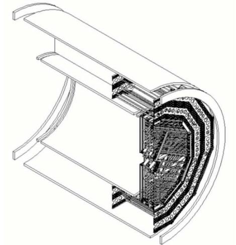
Figure 31: Schematic view of one stave of the barrel muon spectrometer and one end cap. Only a few tubes have been drawn.
