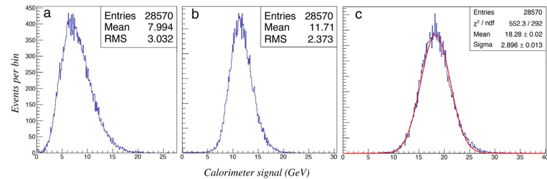
Fig. 11. Signal distributions for 20 GeV  $\pi^-$  particles. Shown are the measured Čerenkov (a) and scintillation (b) signal distributions as well as the signal distribution obtained by combining the two signals according to Eq. (2), using  $\chi = 0.45$  (c).
