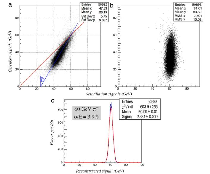
Fig. 14. Signal distributions of the RD52 Dual-Readout lead/fiber calorimeter for 60 GeV pions. Scatter plot of the two types of signals as recorded for these particles (a) and rotated over an angle  $\theta = 30^\circ$  around the point where the two lines from diagram a intersect (b). Projection of the latter scatter plot on the x-axis (c).
