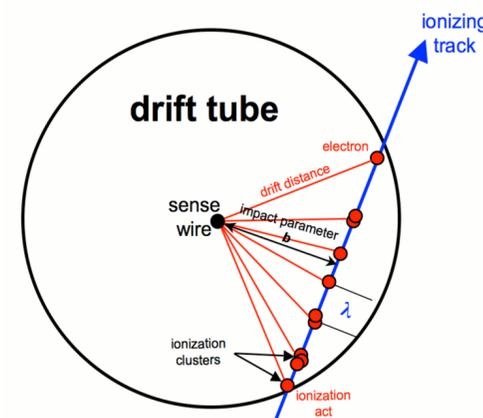
Figure 5: Schematization of the cross view of a drift tube with the definitions used in the text.
