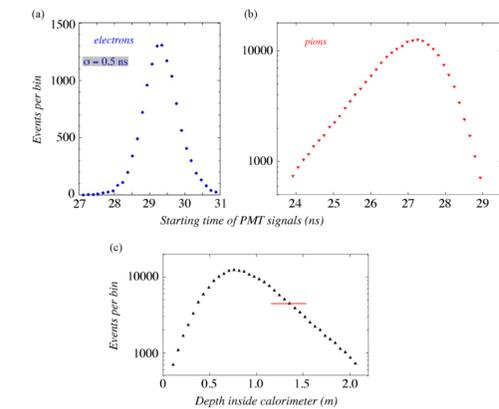
**Fig. 9.** The measured distribution of the starting time of the calorimeter's scintillation signals produced by 60 GeV electrons (a) and 60 GeV pions (b). This time is measured with respect to the moment the beam particle traversed trigger counter T1, installed upstream of the calorimeter (see Fig. 4). These data were used to determine the distribution of the average depth at which the light was produced in the hadron showers (c).
