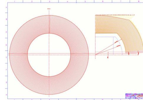
Figure 22: Azimuthal segmentation of the hadronic calorimeter at  $z = 0$ . There are 256 towers in each of the 32 slices in  $\theta$ . At left the  $r - z$  projection, where one can see the segmentation of 32 concentric tower arrangements of the end cap. In blue are the contours of the CluCou chamber. The space between the chamber and the fiber calorimeter is filled with the crystal (EM) calorimeter.
