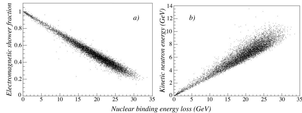
**Figure 6.** The correlations between the binding energy loss and the em shower fraction (a), and the neutron kinetic energy (b) obtained from GEANT 4 simulation in the case that 100 GeV pions produce hadron showers in the lead absorber.
