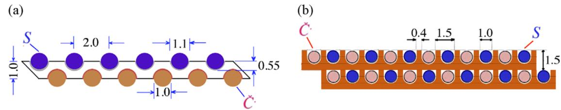
Fig. 3. Basic structure of the new lead (a) and copper (b) based RD52 fiber calorimeters.
