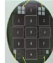
AC-coupled Single- sided strip sensor
