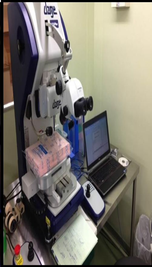
Bonding pull test - Checking pull force
