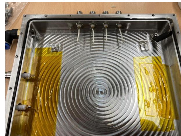
3) Cable soldering on BNC connectors and GND spot
