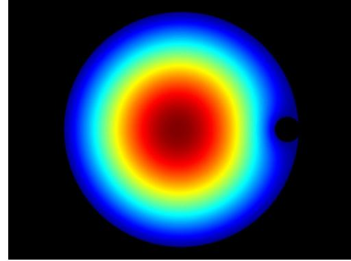
*Conductor rod (TM<sub>010</sub>)*
