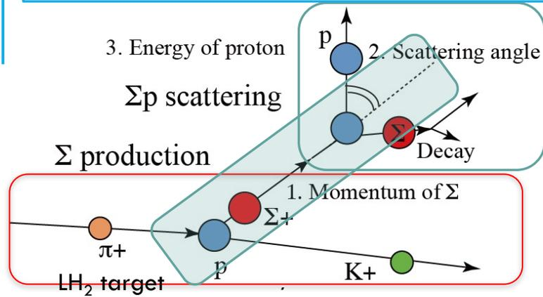
Detection of  $\Sigma p$  scattering event by CATCH detector
