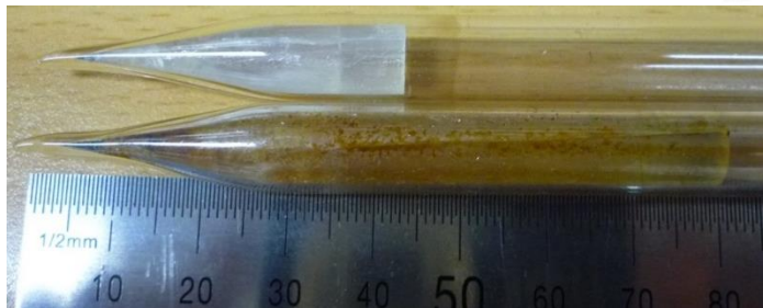
Crystal is growing in Bridgman furnace
